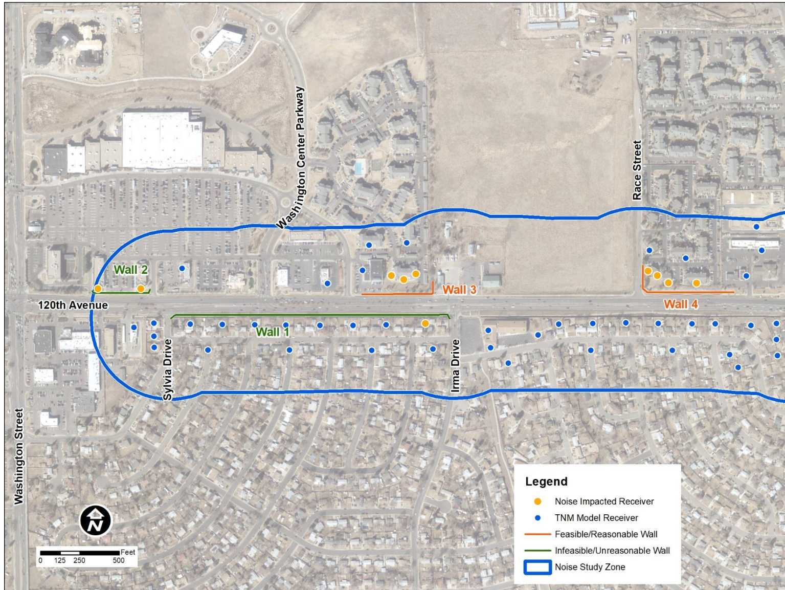
Figure 5 Potential Noise Abatement Barrier Locations and Findings
